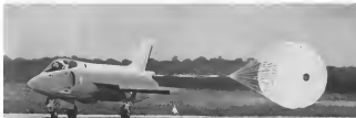
PARADIGM STREAMING rolled behind the Breguet Tuois (lower) with to stop on the concrete strip at Brétigny. Although eyesight is not required for operation from unprepared fields, most of the trials have been conducted from concrete runways.
